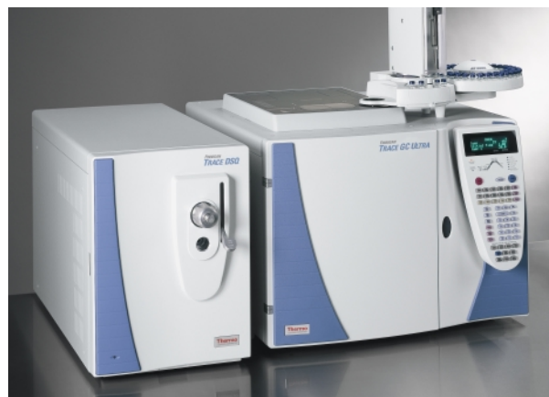
Figure 1. The Finnigan TRACE DSQ is shown with the AS 3000 Autosampler.
